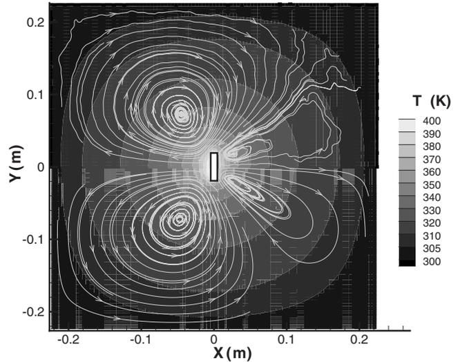
FIG. 4. DSMC (top) and ES-BGK (bottom) streamlines and temperature field in helium.
