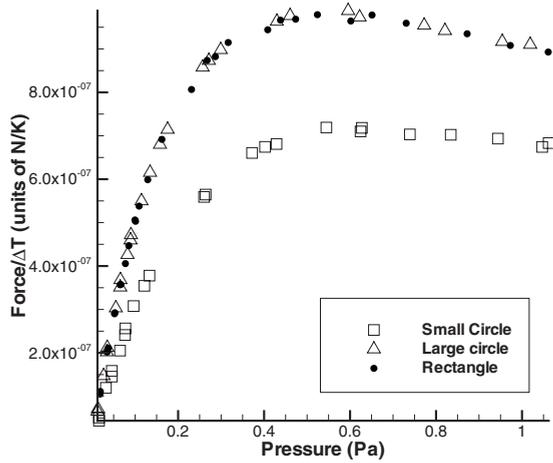
FIG. 2. Measured force on three different plates in argon.
